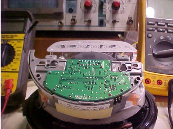
RF Transmitting Analog Meter Circuit Board Removal
